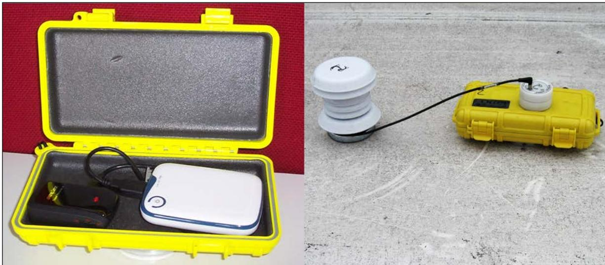
Fig. 6 Mobile measurement campaign in Hamburg. Left: Qstarz BT-Q1000XT GPS logger and Mobile Power Pack VT-PP-320b packed in the waterproof OtterBox 3000. Right: The instrumentation on the roof of a public transport bus. The logger is glued onto the OtterBox, the sensor is inside the radiation protection housing.
