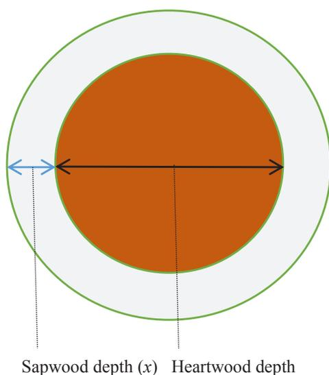
Fig. 1 Sapwood and heartwood of the tree stem (the grey colored part in the edge is the sapwood, the brown colored part in the center is the heartwood). Source: Own elaboration
