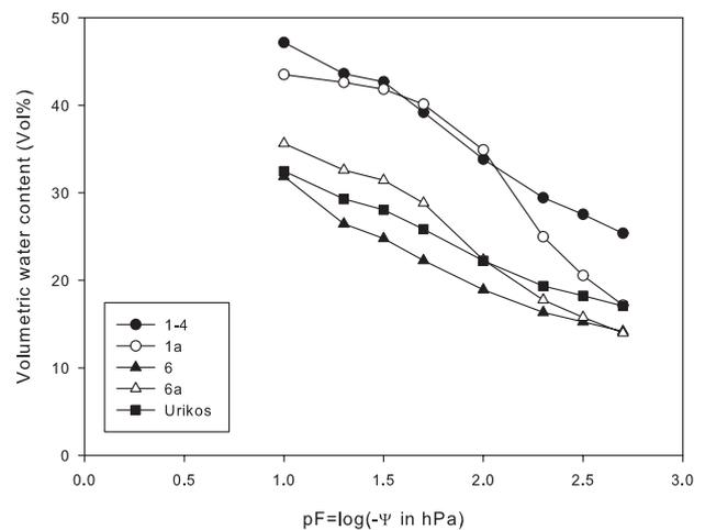
*Fig. 9* Volumetric water content of samples from 2014 as a function of pF at pF 1, 1.3, 1.5, 1.7, 2, 2.3, 2.5, 2.7. Source: own drawing
