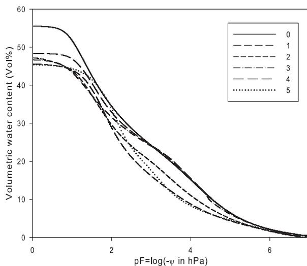
*Fig. 8* Modelled topsoil (ca. 5–10 cm depth) water retention curves for plots 0 to 5 based on data measured with HYPROP and WP4C. Model predictions are based on the PDI-variant of the bimodal unconstrained van Genuchten model and for two samples on the bimodal unconstrained van Genuchten-Mualem model (see text for details). Source: own drawing
