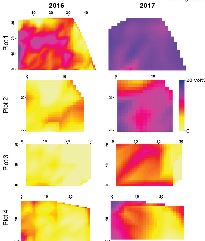
Fig. 7 Soil moisture (Vol-%) at the surface in plots 1 to 4 (given in m) measured in October 2016 (left) and March 2017 (right). The interpolation method applied is triangulation using the mean of three measurements per spot. Note that the moistest spots are  $\geq 20$  Vol-%, the generalized scale allows for comparison among plots and years. Source: own drawing
