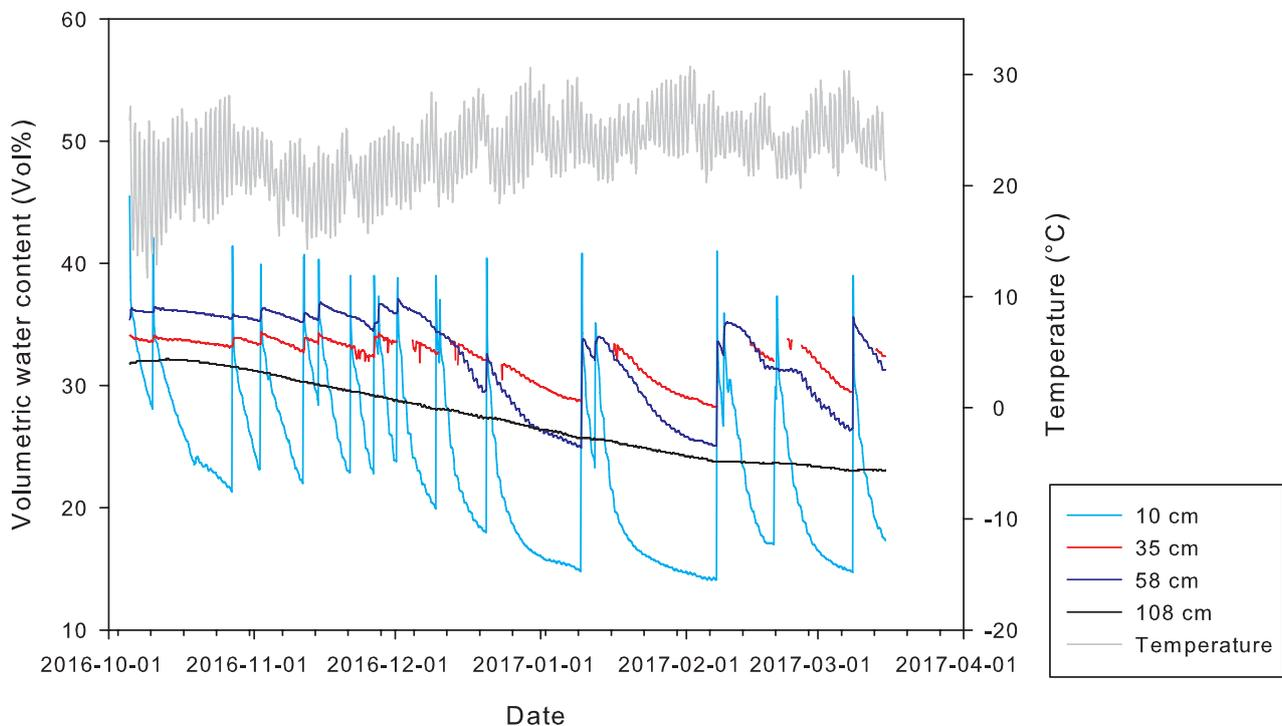
Fig. 6 Volumetric soil moisture in  $\text{cm}^3/\text{cm}^3$  measured in four depths and soil temperature ( $^{\circ}\text{C}$ ) at  $-10$  cm as recorded in plot 3 from October 2016 to March 2017. Source: own drawing
